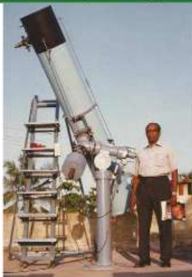
P. Devadas on the roof terrace of his house at Guindy, Madras, India in 1993 with the 355mm telescope that he constructed himself. The main mirror is f/8, and the polar axis shaft is 10cm in diameter.
